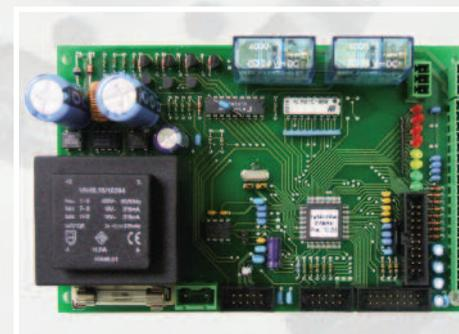
Frequency converter control board. It contains the entire brain of the adjustment control in the form of a microcontroller programme.
