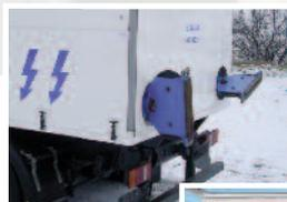
The large cable guide rollers increase the service life of the cable noticeably.
